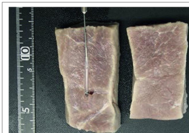
FIGURE 8 | (A) Images of an incised porcine muscle tissue in which a CL target capsule consisting of a 0.5 mm silicone tube, was embedded. (B) Two-dimensional tomographic image obtained with the slab of porcine muscle. The tissue, measuring 50 mm (X) × 50 mm (Y), had a CL target embedded within it to a depth of 25 mm. Reproduced with permission from Kobayashi et al. (2016).
