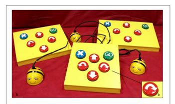
FIGURE 3 | (a) Switched on/off sensors of 65 mm diameter, Jelly Bean; (b) The adapted Bee-bot.
