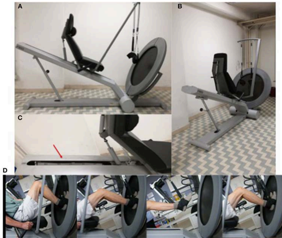
FIGURE 1 | (A,B) Trampoline Trainer exercise device. (C) The red arrow points to the meter scale applied to the rail track of the TT device. (D) Representation of a bounce sequence performed by an elderly volunteer.
