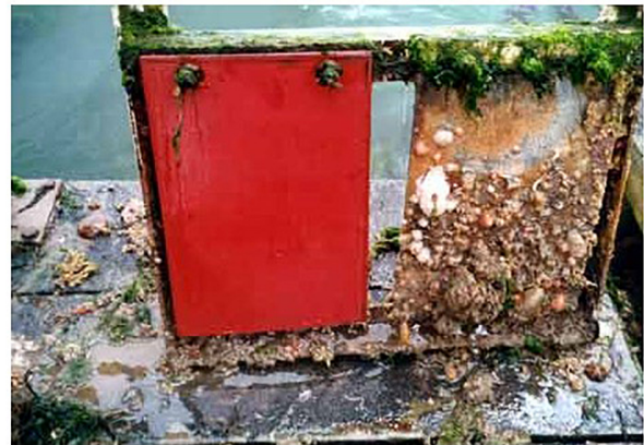
FIGURE 1 | Tributyltin treated ( left ) and untreated ( right ) marine exposed during 1 month.
