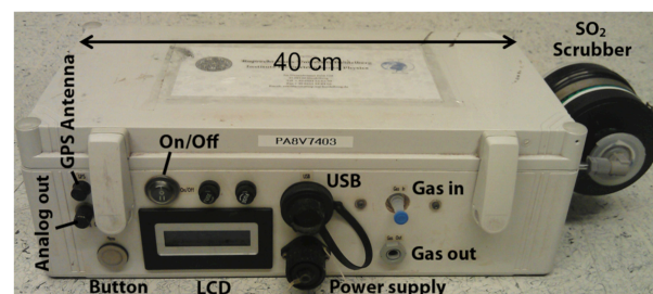
FIGURE 3 | Exterior view of the PITSA instrument. The front panel features: gas in- and outlet, on/off switch for main power (with protective fuses to its right), an LAD screen showing preliminary real time data ( \text{SO}_2 , \text{CO}_2 , temperature and pressure), a programmable push button (typically used to manually trigger zero point measurements) and connectors for USB (real time digital data output, firmware programming), power (battery charging and external power supply), external GPL antenna and analog output (2 channels for \text{SO}_2 and \text{CO}_2 for application with analog data loggers).
