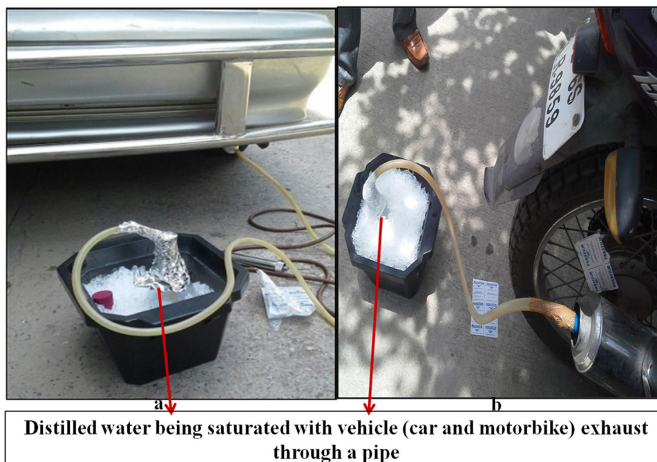
FIGURE 2 | Exhaust fumes from the petrol driven car and motorcycle were collected by connecting one end of a plastic pipe to the exhaust of the car and the other to saturate distilled water (DW) kept in ice bath for an hour which served as a source of CO 2 (adopted from Faridi and Satyanarayana, 2016a).
