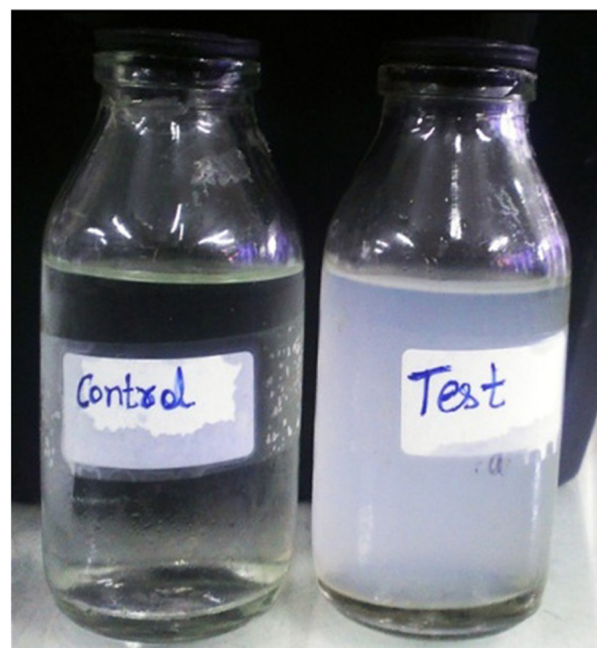
FIGURE 3 | Mineralization of vehicular exhaust gas CO 2 using BhCA in the presence of Ca 2+ . Test reaction containing CA showed efficient mineralization of CO 2 as compared to the control (adopted from Faridi and Satyanarayana, 2016a).
