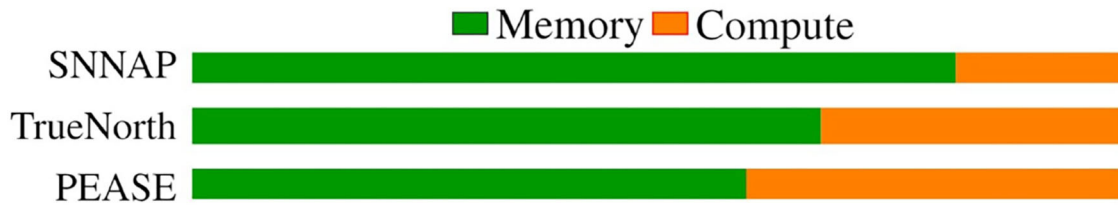
FIGURE 2 | Ratio of memory to compute energy on PEASE, TrueNorth, and SNNAP.
