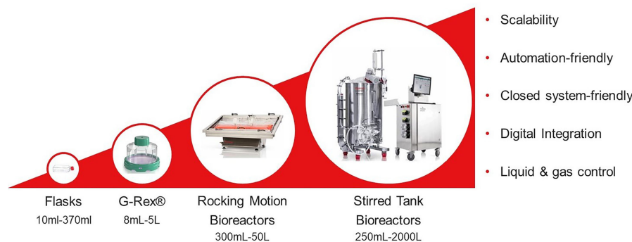
FIGURE 4 | Bioreactors offer several advantages to the clinical manufacturing of cell therapies. The shift from static vessels on the left toward dynamic bioreactors on the right allows for several process improvements, such as scalability, automated and closed operation, digital integration, and intimate control of liquids. These capabilities result in increased safety and consistency, reduced labor requirement and cost, and improved quality of cellular output.
