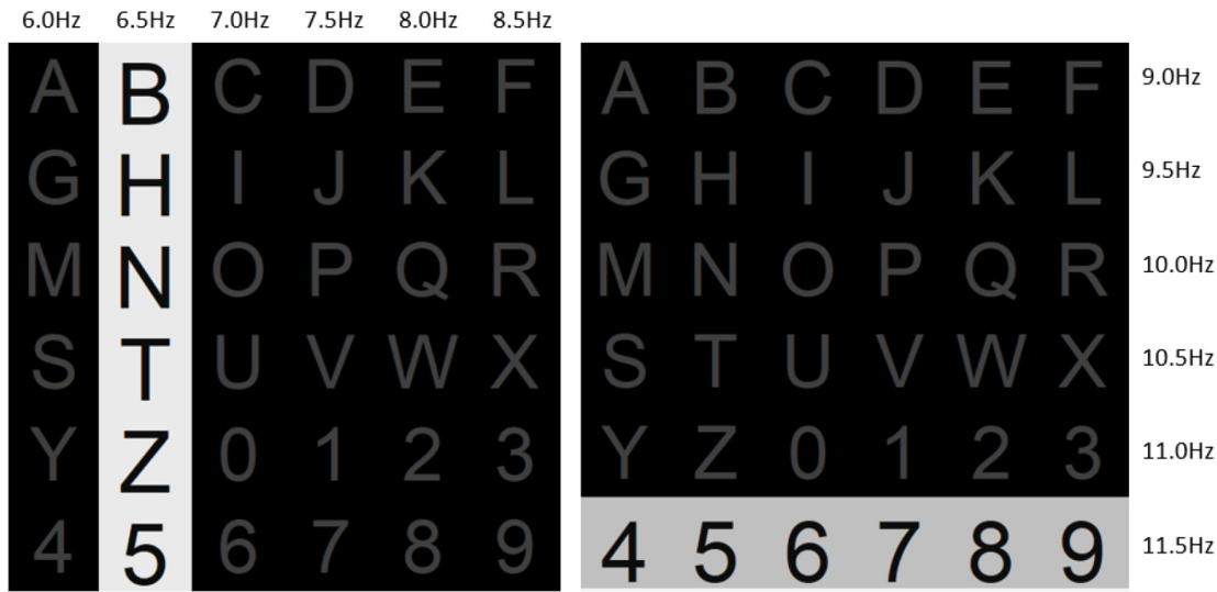
FIGURE 1 The proposed frequency enhanced row and column stimulus paradigm. A flicker (white-black) with a specific frequency is assigned to one row or column of a 6 × 6 layout, and the row/column flashes are carried out in a pseudorandom sequence. In this figure, Column 2 and Row 6 are activated, and the target output is the number “5”.
