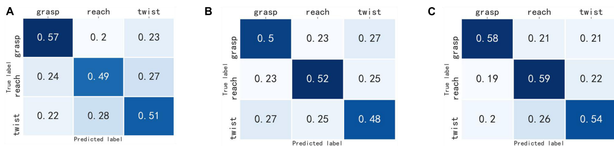
FIGURE 6 Confusion matrix of the three-class classification experiment. (A) EEG-CNN, (B) TF-CNN, (C) MF-CNN.
