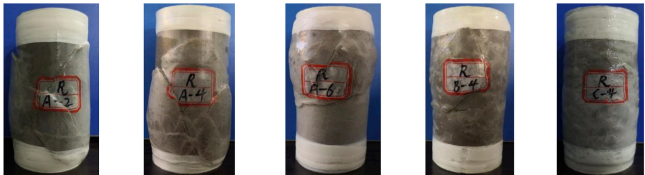
FIGURE 2 Specimens for unloading confining pressure creep test under seepage.
