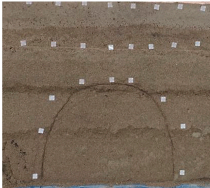
FIGURE 2 | Similar material model and measuring point layout (model front).
