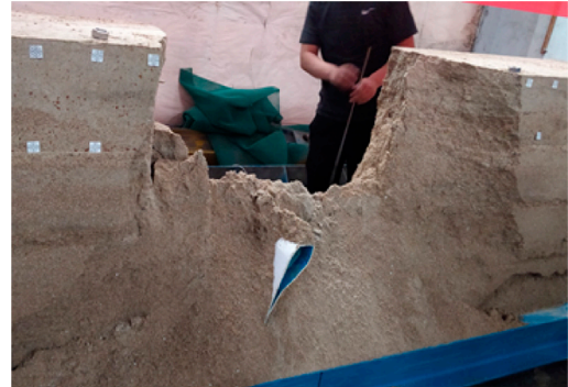
FIGURE 4 | Real picture of tunnel collapse and even surface collapse.
