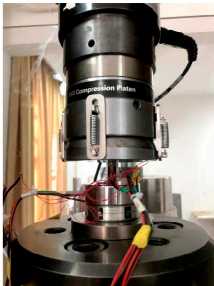
FIGURE 12 | Uniaxial compression test of a granite specimen on a MTS 815 system.
