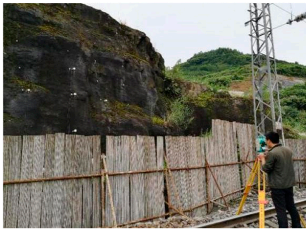
FIGURE 11 | Field measurement using a total station instrument.
