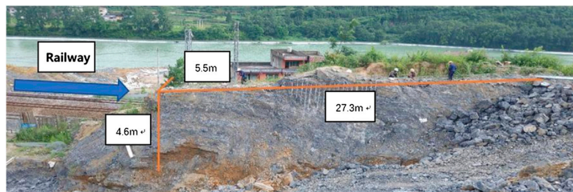
FIGURE 8 | Rock wall site for demolition blasting test.
