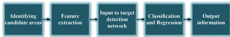
FIGURE 2 | Detection flow of the target identification algorithm (TIA).
