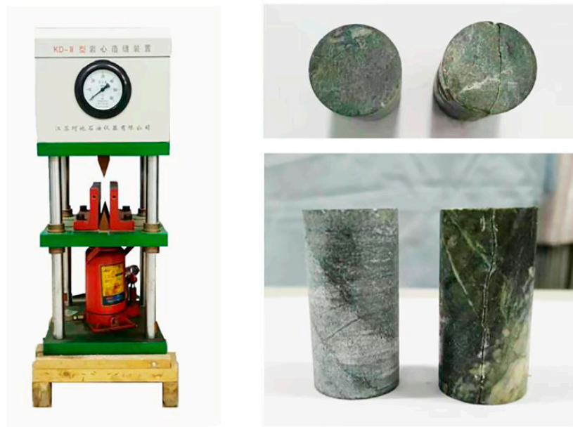
FIGURE 3 | Device for artificially creating fractures and cores before and after splitting.
