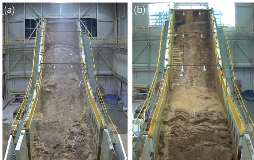
FIGURE 4 | Images of the slope failure after each experiment: (A) first and (B) second experiments.
