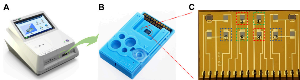
FIGURE 1 | GMR immunoassay analyzer (A), the polymer assay cartridge (B), and the GMR sensor array chip (C). The two selected sensor units used for CRP detection are marked in blue squares (① and ②). The two selected sensor units used for PCT detection are marked in red squares (③ and ④). The two selected sensor units used for NGAL detection are marked in green squares (⑤ and ⑥).
