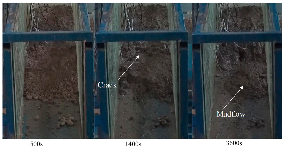
FIGURE 9 | Failure process in the experiment with a slope angle of 17^\circ .
