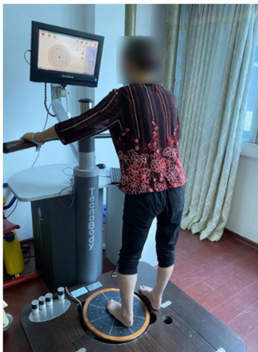
FIGURE 1 | Participant used the Pro-kin system to test the lower limb proprioception.
