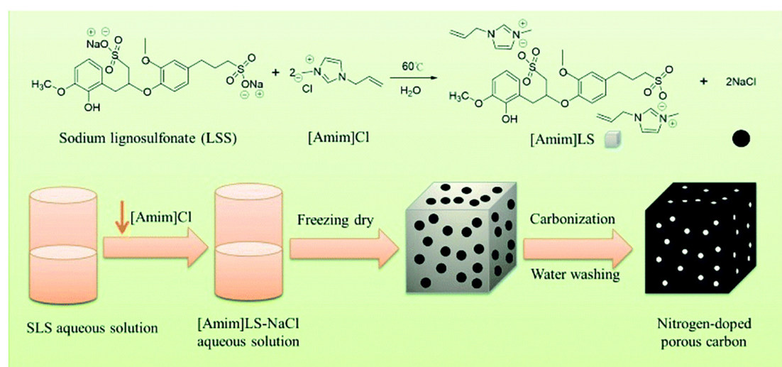
FIGURE 5 | Schematic diagram of [Amim]LS precursors for N-doped porous carbon material fabrication (Xu Q. Q. et al., 2020).
