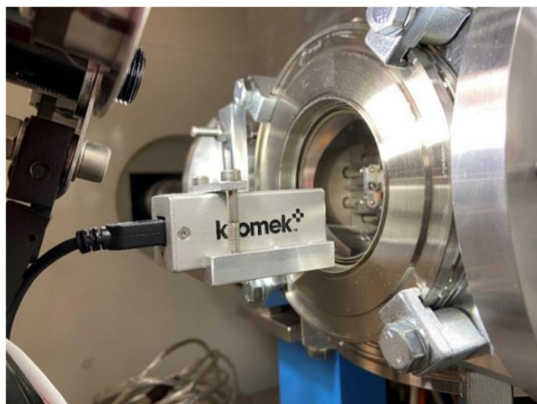
FIGURE 7 | CZT \gamma -ray detector installed in front of the window of the collection chamber and performing the on-line measurement of the activity being implanted on the foils.
