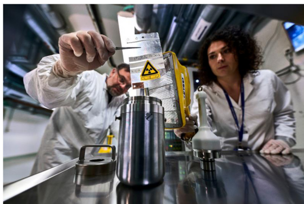
FIGURE 4 | Dose rate measurement on the first collection of Tb-155 at CERN-MEDICIS.
