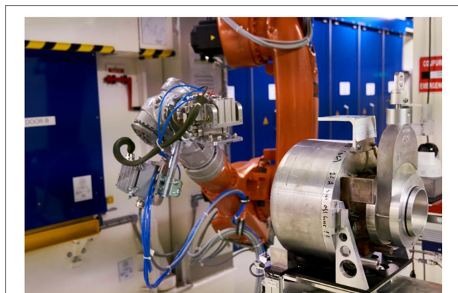
FIGURE 2 | The MEDICIS robot about to transfer a target from the RCS to the target station.
