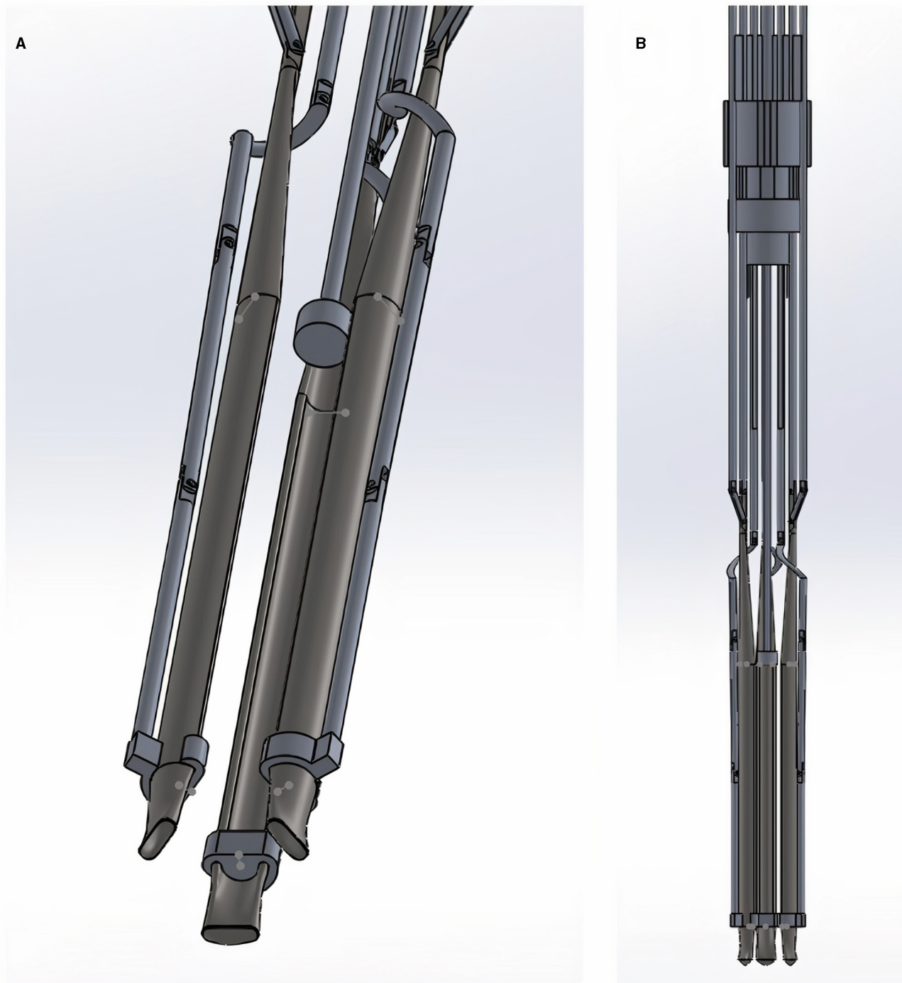
FIGURE 2 | (A,B) Close-up angled view (A) and complete lateral view (B) of the distal end of the instrument (the patient end where the patch would be enclosed). Movements of this compartment are controlled at the other (operator's) end of the instrument by the connected Grips shown in Figure 1 .
