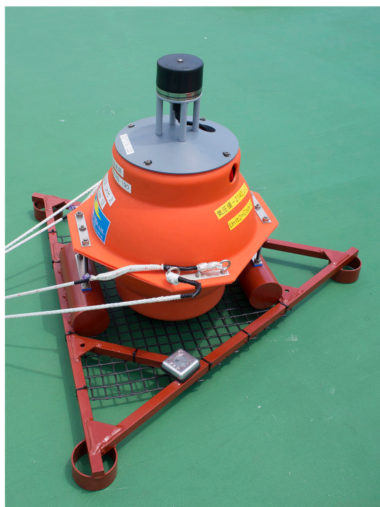
FIGURE 4 | Photo of an ocean bottom acoustic transponder installed in the test site. The black device fixed on the top is the acoustic transducer.
