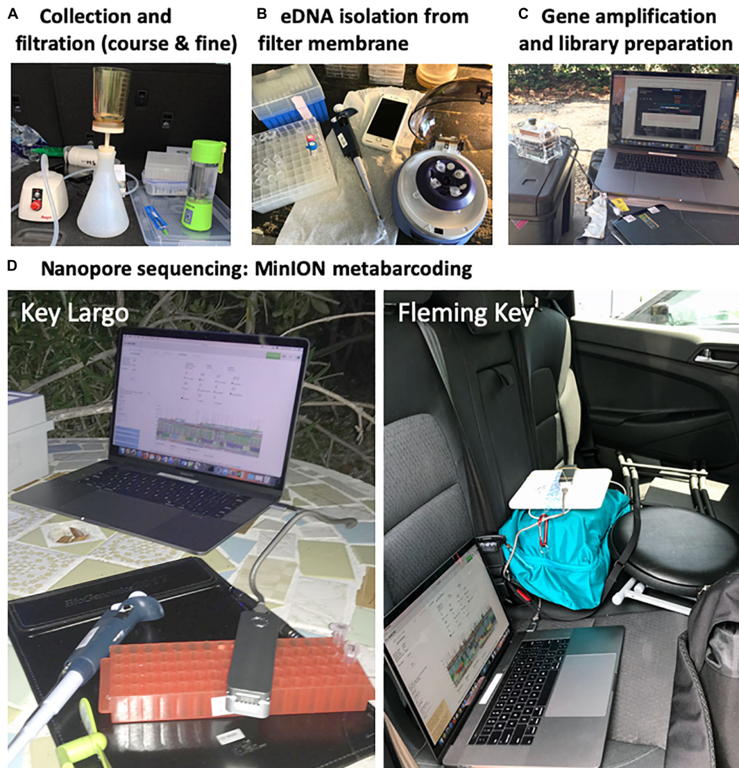
FIGURE 2 | Overview of FeDS workflow used in this study for collection sites in both Upper Keys (BC01 – BC04) and Lower Keys (BC05 – BC08). (A) Triplicate seawater samples were collected from each sampling location and processed in the field within 1–2 h post-collection. Coarse filtration was conducted, followed by homogenization and fine filtration on a water-testing membrane filter. (B) Filter membranes (containing eDNA filtrate) were kept in buffer at ambient temperature until eDNA was extracted; in the final step, isolated eDNA was concentrated in 70 \mu l of elution buffer. All equipment was sanitized between stations. (C) Molecular protocols including PCR were carried out using an USB-operated 8-well thermocycler (miniPCR). (D) Nanopore sequencing metabarcoding with MinION commenced in Upper Keys (BC01 – BC04) outside on a bluff overlooking Buttonwood Sound, and in Key West (BC05 – BC08) in a rental car.
