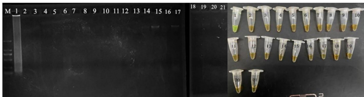
FIGURE 1 | Specificity of CPA detection for different strains with pheS genes by 1.5% agarose gel electrophoresis and mixed chromogenic agent; M-DNA marker; lane/tube 1, P. acidilactici BM-PA17927; lane/tube 2–20, non- P. acidilactici BM-PA17927 strains of E. coli , Salmonella enteric , Vibrio parahaemolyticus , Pseudomonas aeruginosa , Listeria monocytogenes , Staphylococcus aureus , and Lactobacillus casei ; lane 21, negative control.
