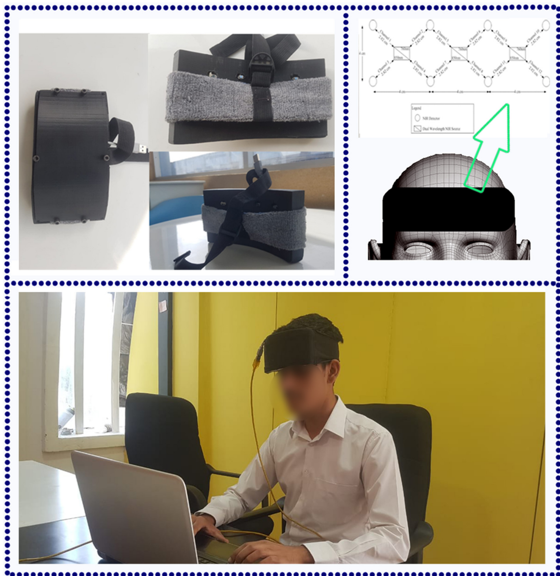
FIGURE 2 | The functional near-infrared spectroscopy (fNIRS) (P-fNIRSSyst) system placed to measure participants' prefrontal cortex (PFC) activity. Optodes are placed according to the standard 10–20 system.
