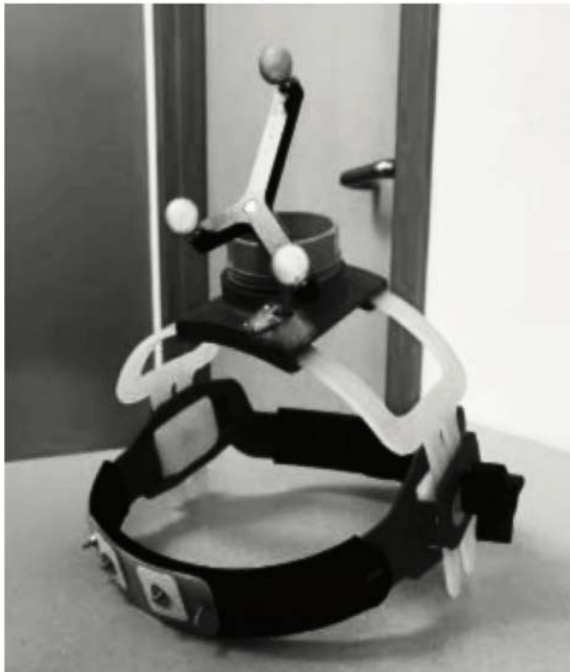
FIGURE 1 | Custom-Engineered tSMS Helmet. Custom designed and partially 3-D printed helmet used for application of tSMS with neuronavigation.
