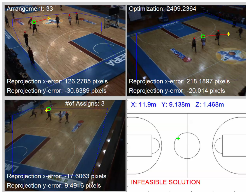
FIGURE 8 | An example of combination tested with re-projection errors detailed. The head detected (red asterisk) that were designed to a given player (green circles) resulting in a poor 3D reconstruction, which the value of re-projection errors (red lines between green circles and yellow plus sign) are too large, and then provide an infeasible solution due to the one constraint.
