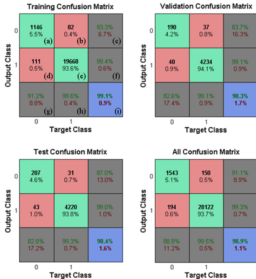
FIGURE 10 | Neural Network classification. Neural network confusion matrices (Matlab confusion matrix plot model), 'head' is 1 and 'non-head' is 0. True classifications are denoted by green squares (a,e) and false classifications are denoted by red squares (b,d). Blue squares indicate the overall rates (correctness and error rate) of classifications (i). Gray squares (c,f,g,h) show the conditional rates (correctness and error rate) given a pre-determined target (3rd row, g,h) or given a pre-determined output (3rd column, c,f). The performance was evaluated in Game 1 for each subset.
