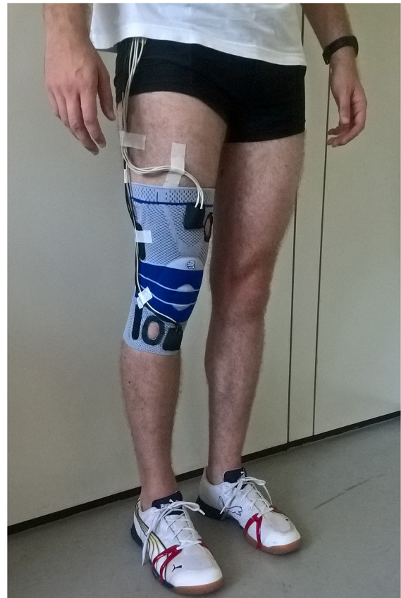
FIGURE 1 | A participant wearing the knee sleeve on the right leg. The two inertial measurement units were placed in the patch pockets at the upper and lower frontal end of the knee sleeve.
