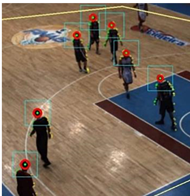
FIGURE 3 | Head candidates' points. Heads enclosed by the Circle Hough Transform (the square around of the heads delimited region for a computation of HOG features).
