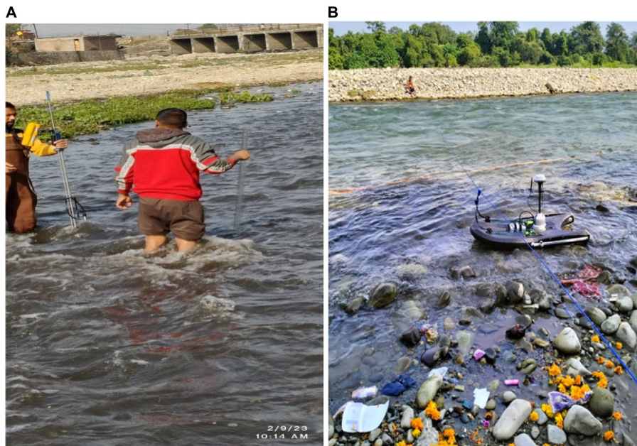
FIGURE 4 Discharge measurement using (A) Flow-Tracker2 in low flow condition (B) ADCP in high flow condition.
