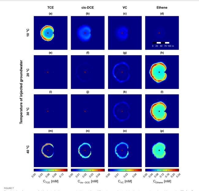
Simulated surface maps of chlorinated ethene concentrations at four different groundwater injection temperatures (rows) (scenarios S3a (a–d), S3b (e–h), S0 (i–l), and S3c (m–p)) at the end of the simulations at 360 days. Red and blue dots indicate the injection and extraction wells, respectively.
