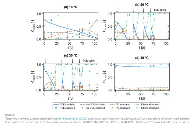
from batch microcosm setups at four different temperatures, (a) 10°C, (b) 20°C, (c) 30°C, and (d) 40°C. Additional TCE was spiked to microcosms operated at 20°C and 30°C after 3, 35, 56, and 70 days (arrows at top of panels **b,c**).
