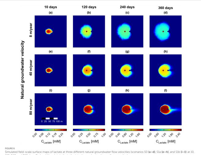
120, 240, and 360 days. Red and blue dots indicate the injection and extraction wells, respectively
