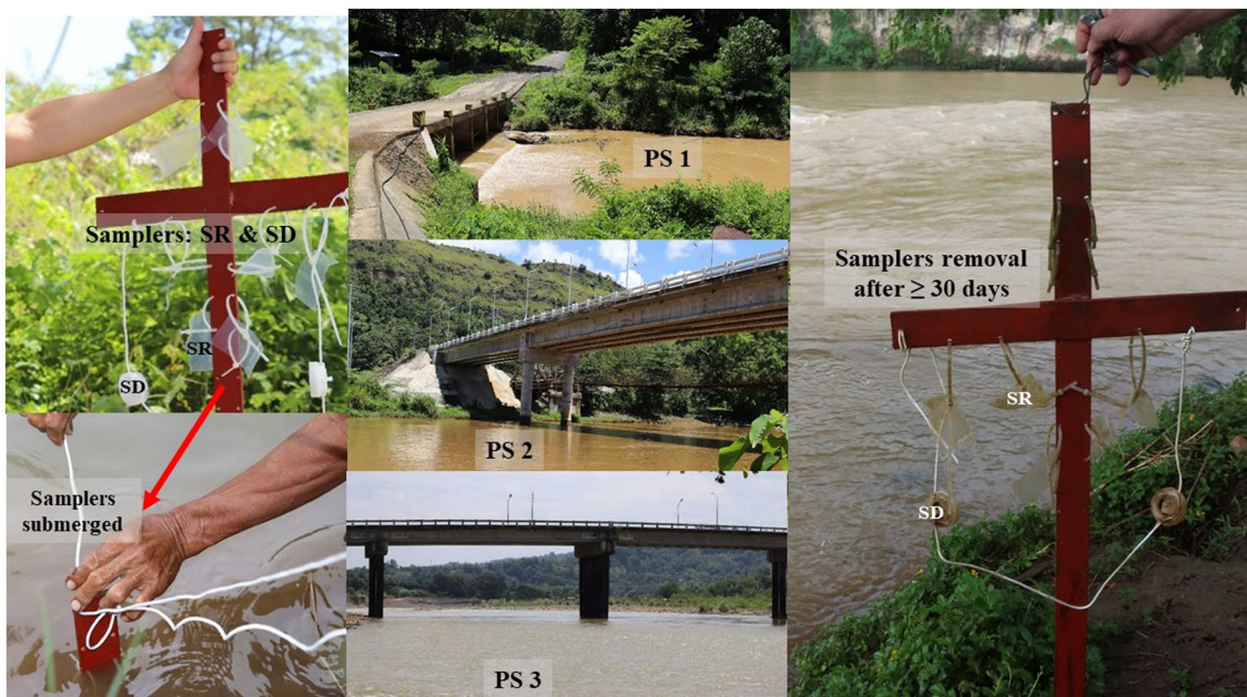
FIGURE 4 Passive samplers composed of six silicone rubbers (SR) and three speedisks (SD) arranged in an iron stand as shown in the upper left picture. The iron stand with the samplers was submerged in river water uninterrupted for at least 30 days as shown in lower left figure. The three middle pictures are the sampling sites; upper is PS1, the middle is PS2, and the lower is PS3. Right picture the removal of iron in preparation for pesticide analyses.
