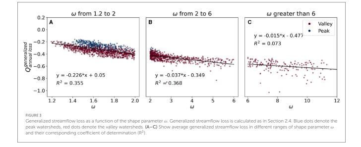
shape parameter of the valley watershed (an average value of 3.1) than the peak watershed (an average value of 1.3). When comparing with the streamflow loss in dry years relatively to normal years, the shape parameter ranges from 1.2 to 2 and from 2 to 6 correlates well with  $R^2$  of 0.355 and 0.368, respectively. The shape parameter
