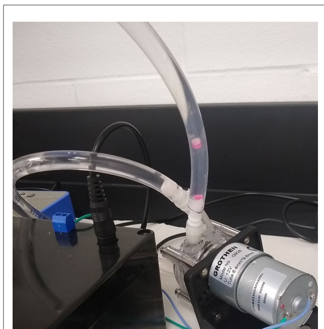
FIGURE 10 Clogging of the connection tubes by the MP particles.
