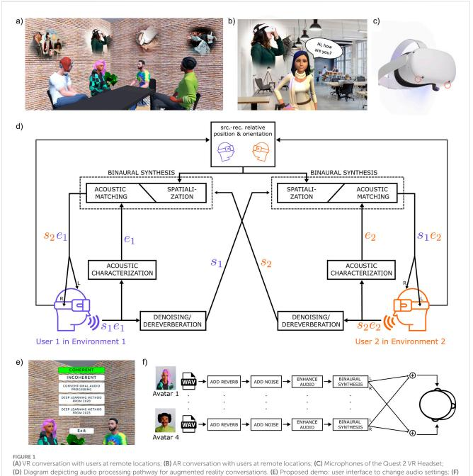
Proposed demo: schematic signal flow.
