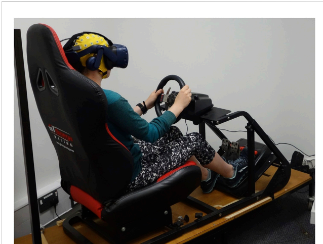
FIGURE 1 Setup of the driving simulator with VR headset and EEG cap.
