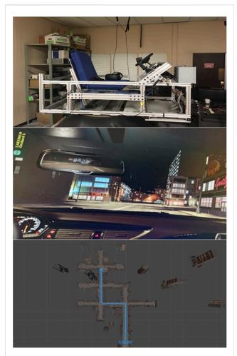
FIGURE 1 VISION Platform, virtual display of participant while using VISION platform and route taken by virtual car during crash route.
