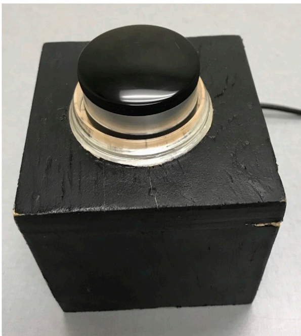
FIGURE 2 Potentiometer knob used by participants to index vection. Photo credit: Ramy Kirolos.
