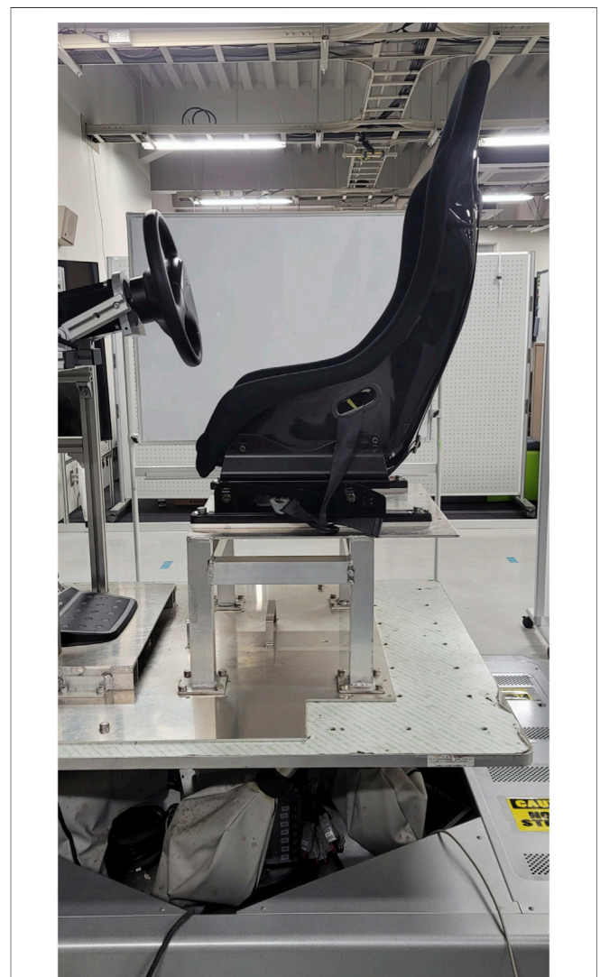
FIGURE 2 | Chair attached to the vibrating device for the experiment.
