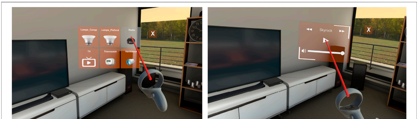
FIGURE 2 | The dashboard interaction mode. On the left the dashboard displays the icons of the six connected objects of the room. On the right, when the icon of a connected object is clicked, its associated user interface is displayed on the dashboard. Here it corresponds to the interface to control the radio.
