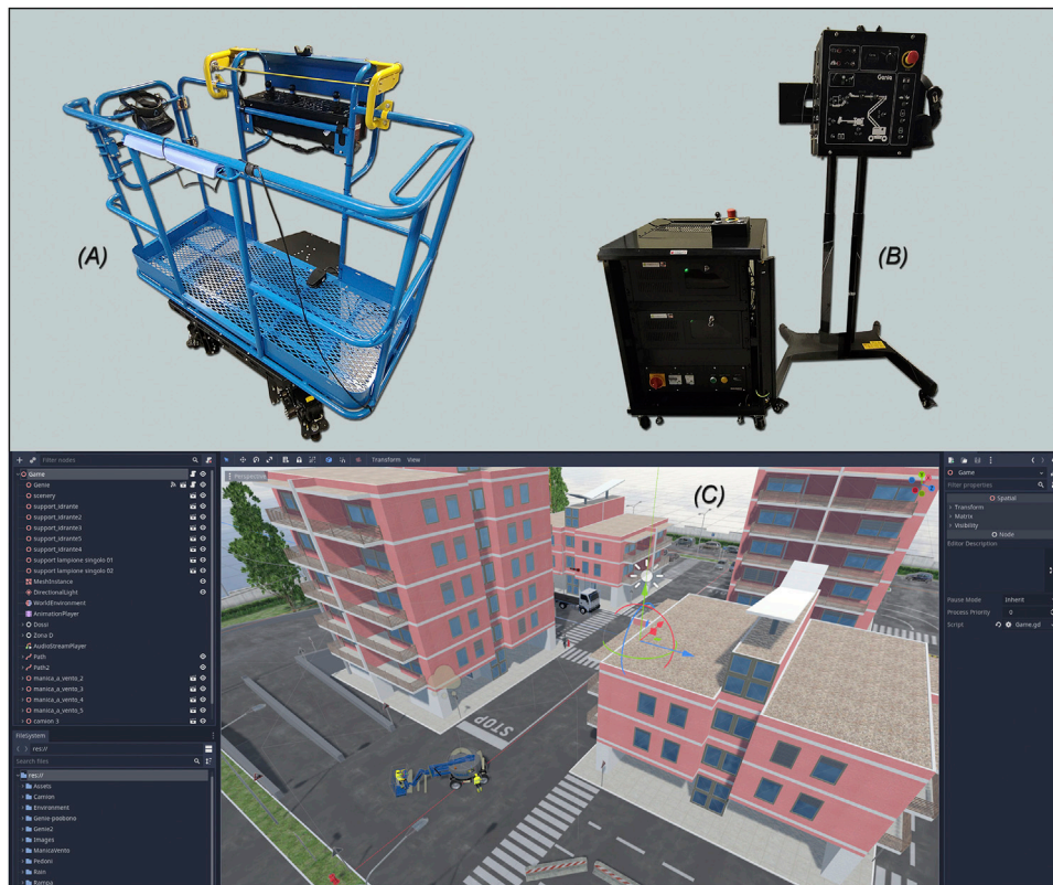
FIGURE 1 The simulator main elements: (A) Aerial platform simulation station; (B) Ground simulation station and computers controlling the simulation; (C) Operating scenario of the simulation.
