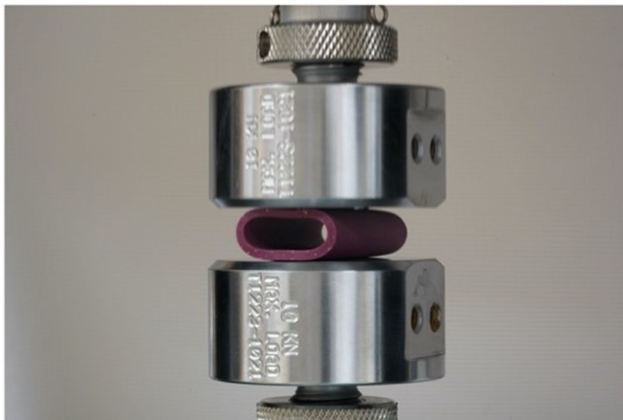
FIGURE 11 Two compression platens mid-compression of silicone stent during mechanical testing.
