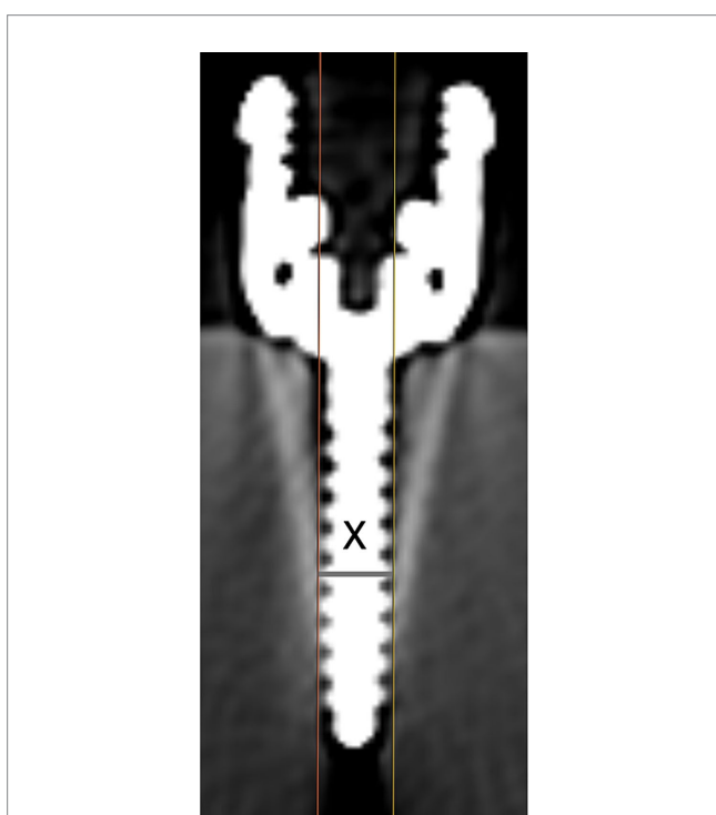
FIGURE 2 Technique to measure screw width, where ‘x’ designates the maximum width for this screw on this slice.
