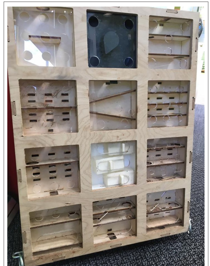
FIGURE 1 | Gorilla Game Lab cognitive enrichment device. A 3D finger maze consisting of 12 puzzle modules. The modular design allows a camera to be fitted inside or on top of the modules. In turn, this allows footage of the gorilla engaging with the device to be recorded.
