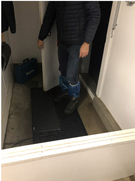
FIGURE 6 Dirty area of the turkey barn (pressure mat and antenna located on the floor)—Maximus prototype.
