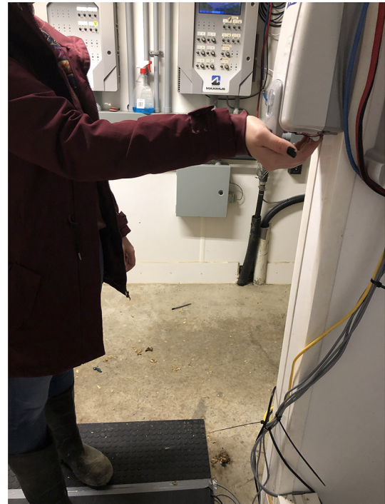
FIGURE 7 Clean area of the turkey barn (pressure mat and antenna located on the floor connected to the hand sanitizer device)—Maximus prototype.
