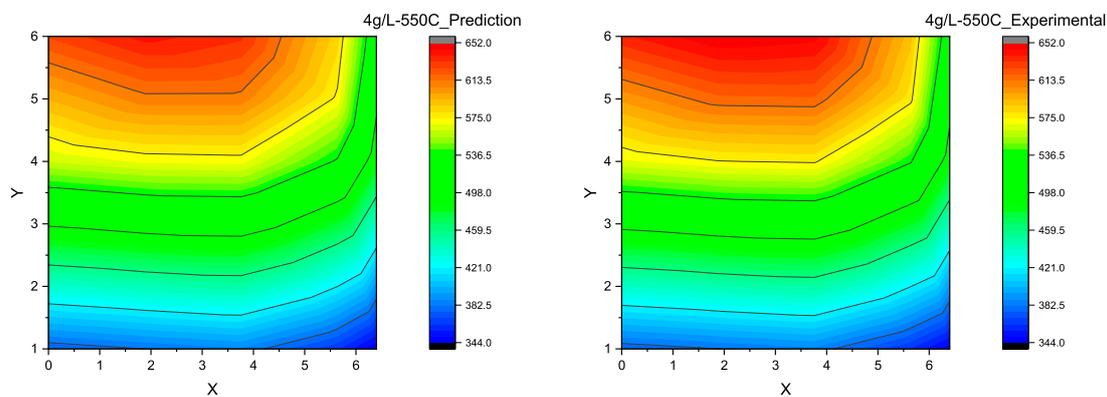
**FIGURE 10** Contour plot for DPF thermal gradient: ANN prediction vs experimental measurement at the soot loading of 4 g/L and the DPF inlet gas temperature of 550°C.
