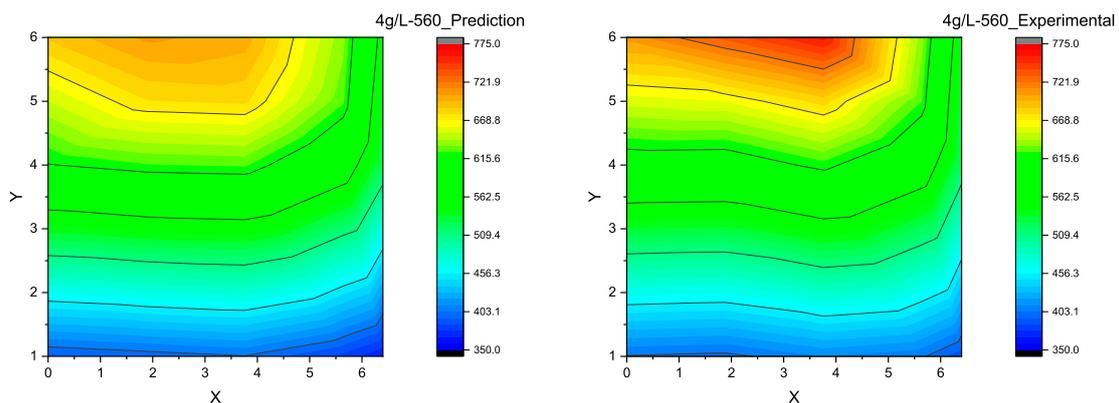
**FIGURE 15** Contour plot for DPF thermal gradient: ANN prediction vs experimental measurement at the soot loading of 4 g/L and the DPF inlet gas temperature of 560°C (Scenario 7 where the experimental data has not been used for the model training and validation, or the so-called unexposed or new data, and the experimental measurement is the field data where the soot distribution may not be as uniform as for the previous scenarios of laboratory tests.).
