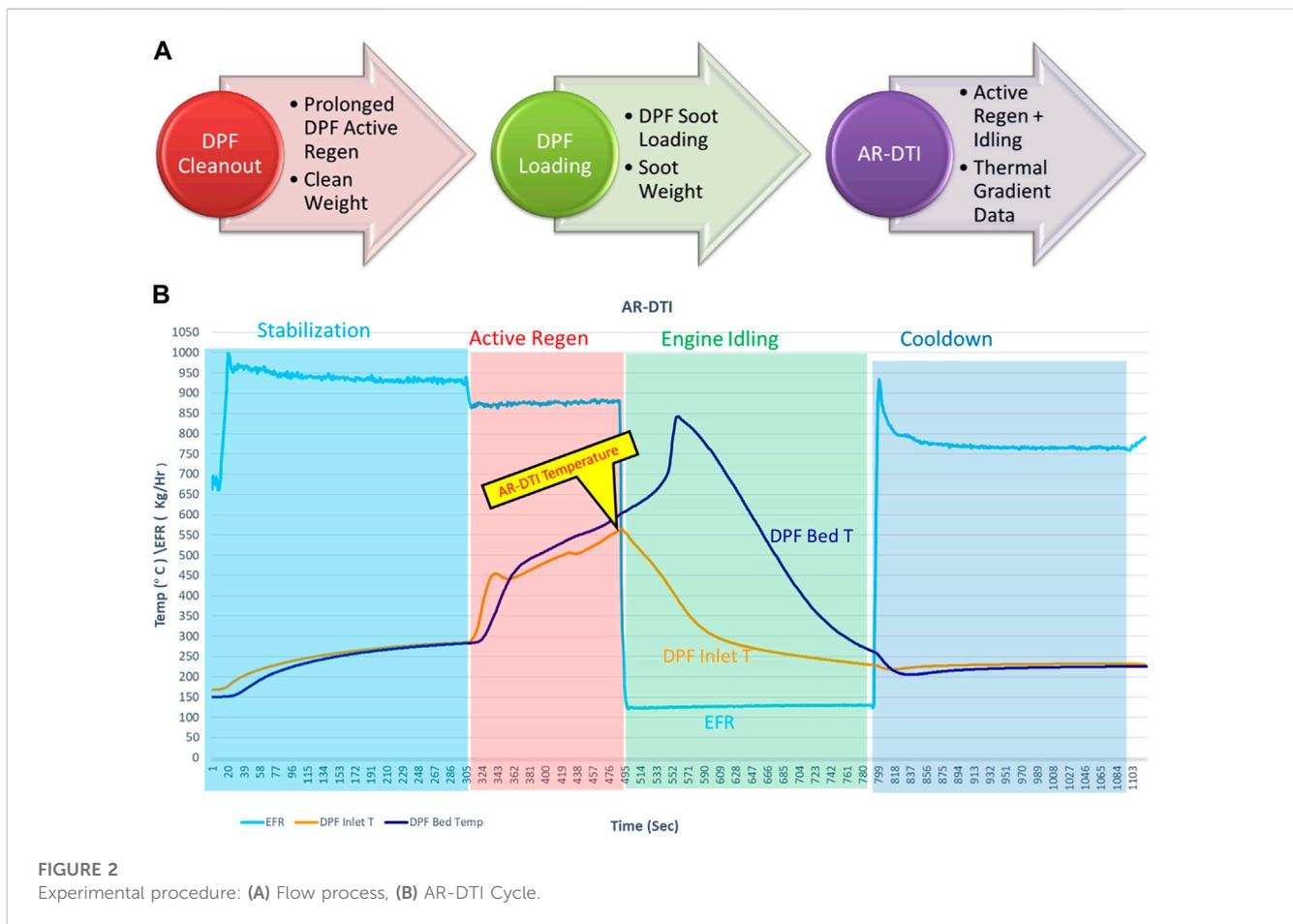
**FIGURE 2** Experimental procedure: (A) Flow process, (B) AR-DTI Cycle.
