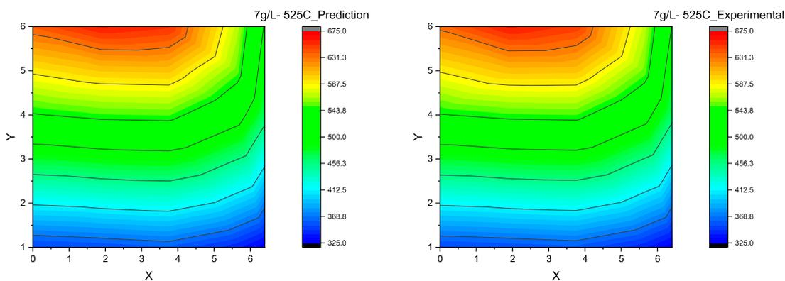
**FIGURE 14** Contour plot for DPF thermal gradient: ANN prediction vs experimental measurement at the soot loading of 7 g/L and the DPF inlet gas temperature of 525°C (Scenario 6).
