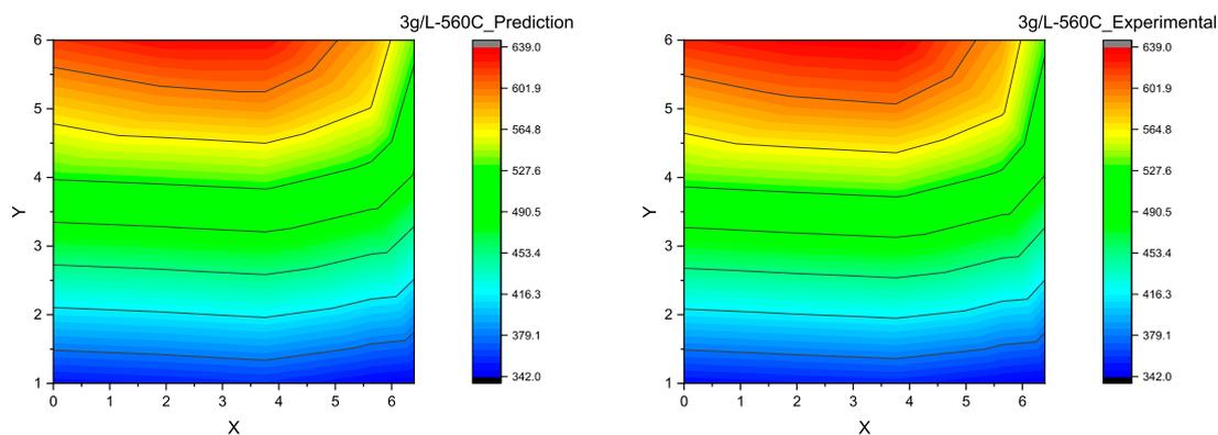
**FIGURE 9** Contour plot for DPF thermal gradient: ANN prediction vs experimental measurement at the soot loading of 3 g/L and the DPF inlet gas temperature of 560°C.
