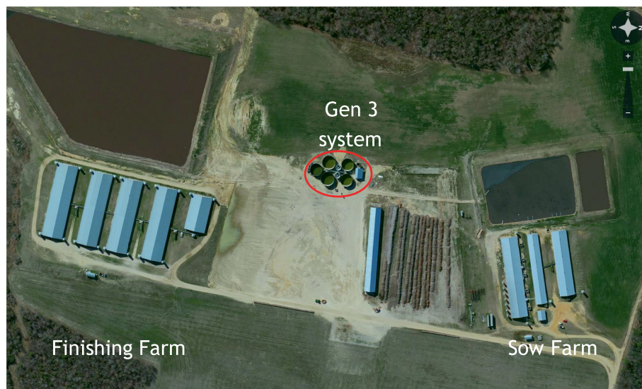
FIGURE 4 Third generation EST swine waste treatment system (red circle) that replaced the lagoon system (existing lagoons shown above the barns) using solid–liquid separation, nitrogen, and phosphorus modules. The new system provided treatment to all the manure from two operations: a 1,200-sow farrow-to-feeder farm that used flushing (right), and a 12,960-head feeder-to-finish farm that used pit-recharge (left).
