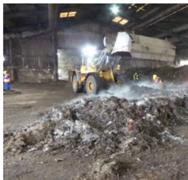
Formation of post-rotting windrow
