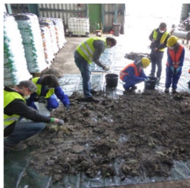
Removal of clearly visible BDP fragments
