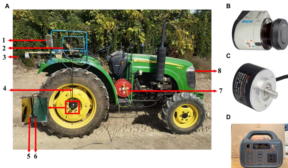
FIGURE 2 Overall layout of test platform and key modules. (A) Overall layout of test platform. Computer power conversion module, 1; Portable computer, 2; Lidar, 3; Encoder fixed frame, 4; Coupling, 5; Encoder, 6; Removable power socket, 7; JOHN DEERE 454 45HP Wheel Tractor, 8. (B) LMS141-15100 two-dimensional Lidar. (C) OidEncoder Absolute encoder. (D) Beeste AS300 mobile power.
