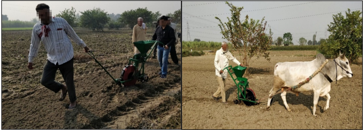
PLATE 3 SRSWI-planter pulled by a human and a bullock.
