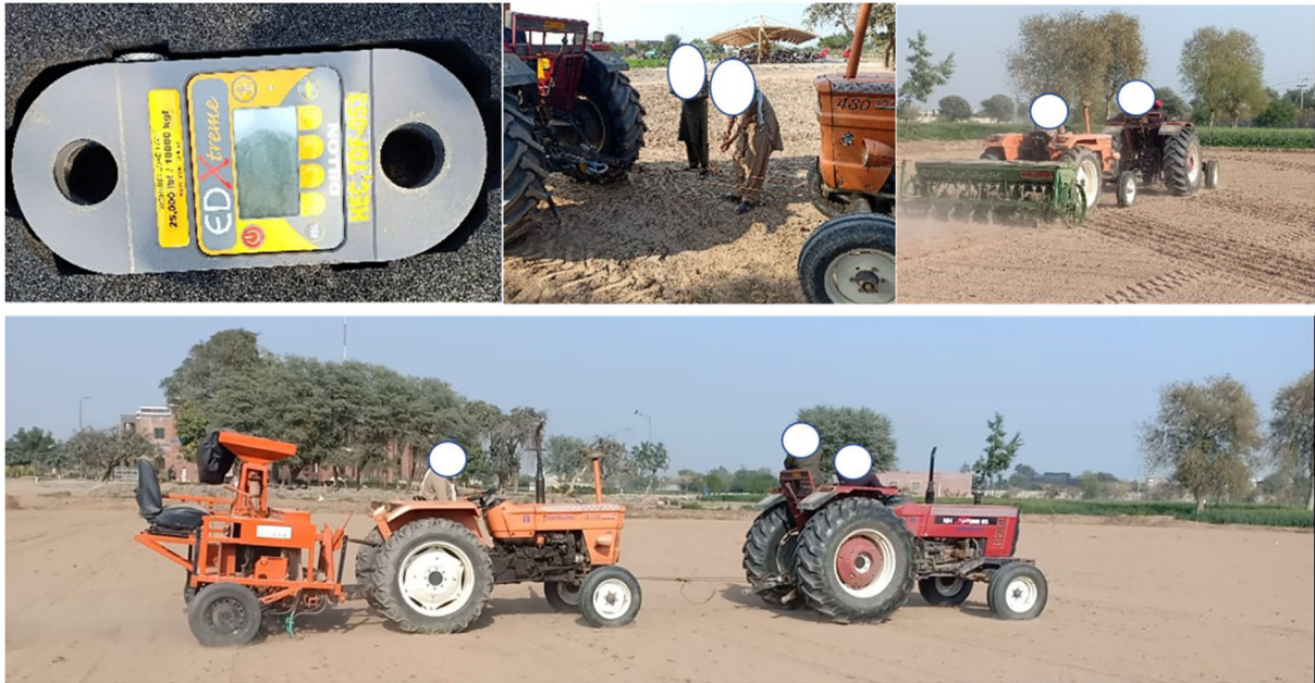
FIGURE 7 Power measurement in field through dynamometer.
