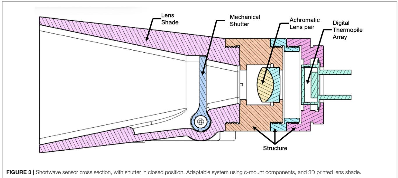
**FIGURE 3** | Shortwave sensor cross section, with shutter in closed position. Adaptable system using c-mount components, and 3D printed lens shade.
