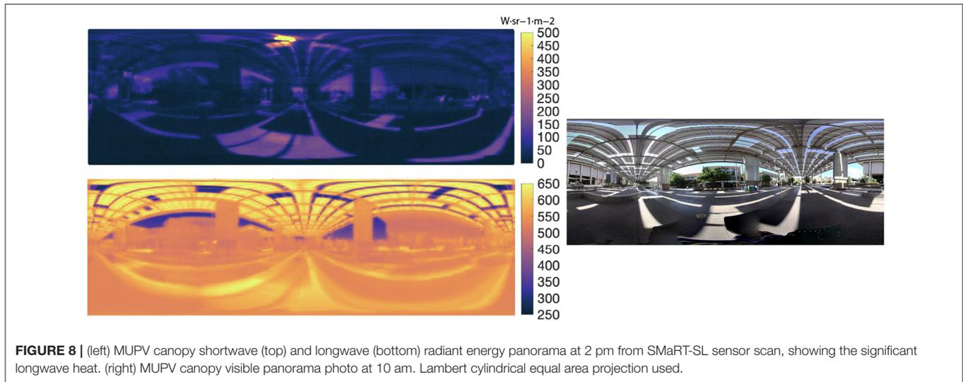
**FIGURE 8** | (left) MUPV canopy shortwave (top) and longwave (bottom) radiant energy panorama at 2 pm from SMaRT-SL sensor scan, showing the significant longwave heat. (right) MUPV canopy visible panorama photo at 10 am. Lambert cylindrical equal area projection used.
