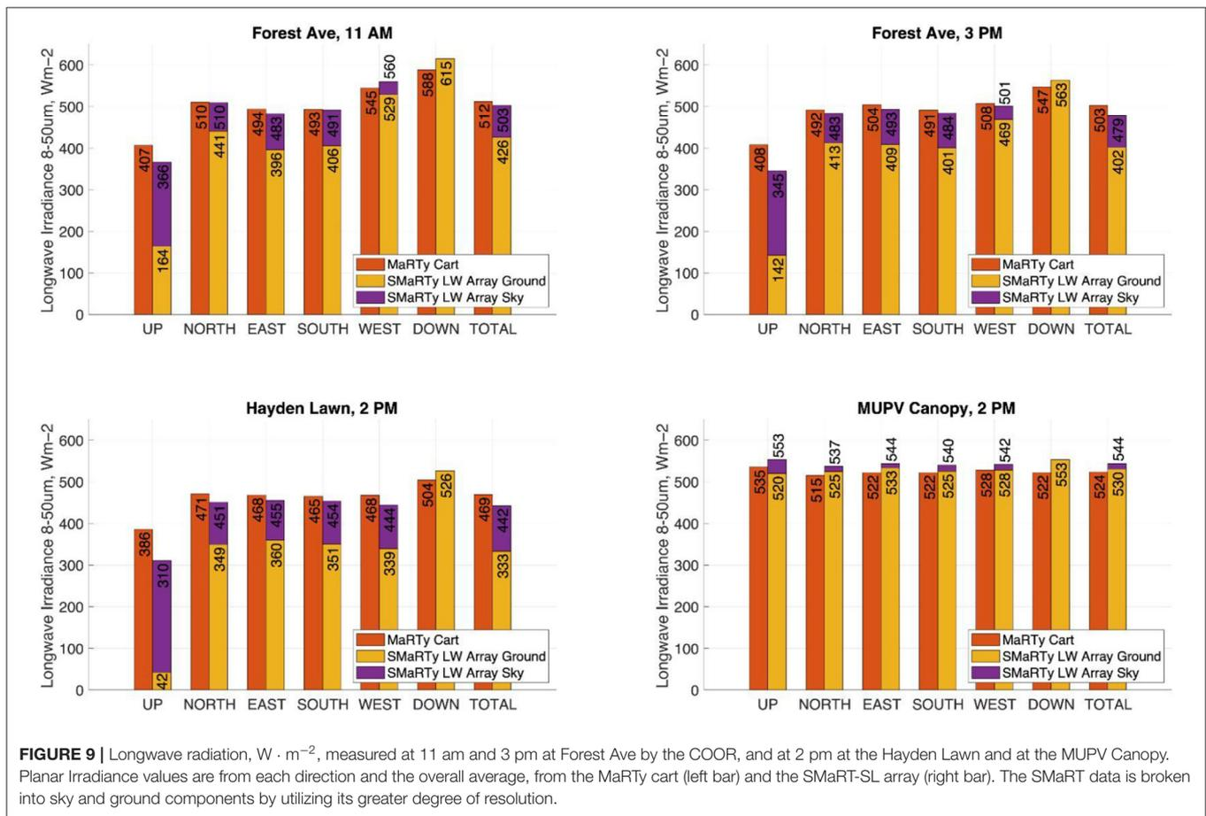
**FIGURE 9** | Longwave radiation,  $W \cdot m^{-2}$ , measured at 11 am and 3 pm at Forest Ave by the COOR, and at 2 pm at the Hayden Lawn and at the MUPV Canopy. Planar Irradiance values are from each direction and the overall average, from the MaRTy cart (left bar) and the SMaRT-SL array (right bar). The SMaRT data is broken into sky and ground components by utilizing its greater degree of resolution.
