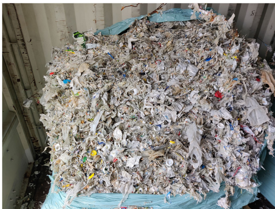
FIGURE 6 LPB repulping reject including mostly PE plastics.
