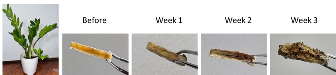
FIGURE 3 Degradation of thermoplastic molded rods in planted soil with 160 mL of room temperature water added each week.
