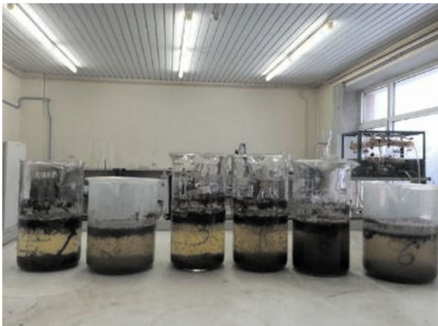
FIGURE 2 Static buoyancy test (12 h).
